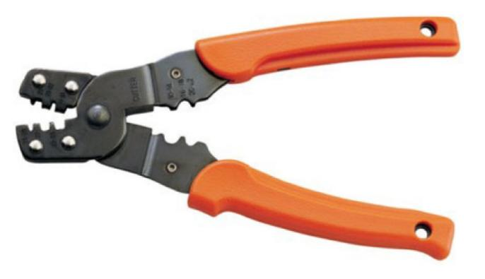
Applicable: Use with the automotive terminals and open barrel terminals.
