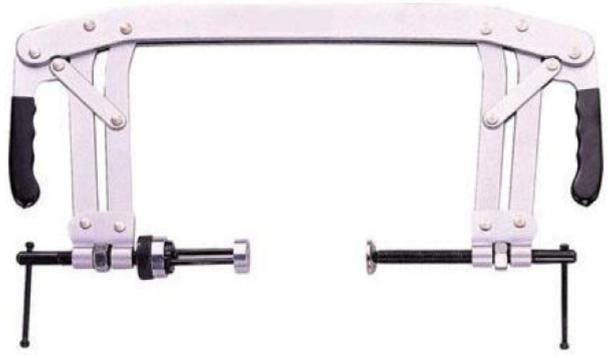
• Suitable for use on multi-valve petrol & diesel engines with deep seated valves.
