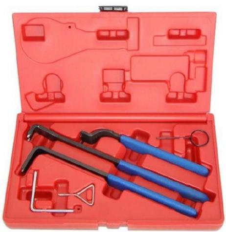
• The belt tensioner roller has two holes in which the two pins of the double pin are inserted allowing them to turn the belt tensioner roller and to tension the timing belt.
