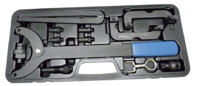
• A complete set for alignment, adjustment the camshaft, replacement the timing chain, etc.
