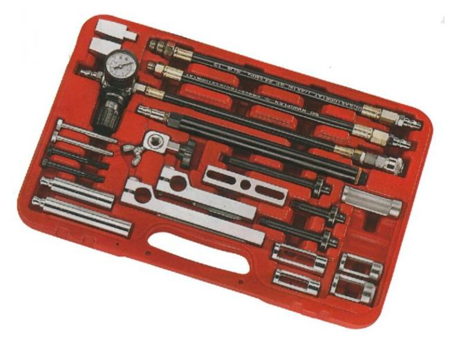
Special designed to remove and install the valve spring and oil seal on various vehicles.
