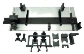
• The essential cylinder head rebulid kit is for VAG and Porsche CR diesel engines.
