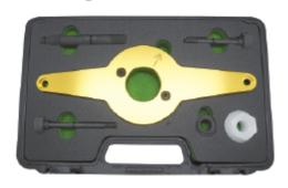
• An essential tool kit required to maintain the engine timng when removing the front vibration
