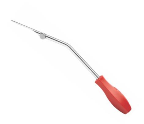
To use, run the wire through the hole at the end of the tool. Then, with the wire on the round side of the tool, attach the end of the wire in the hole midway up the tool, locking it in place with the set screw. Move the tool on the inside of the vehicle, a few inches at a time, while the person on the outside follows doing the cutting. The smooth metal will move under the moldings and along the dash and prevent damage
