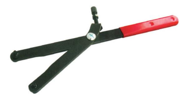
• Keeps flywheel, rotors and sprockets from rotating during removal and installation.
