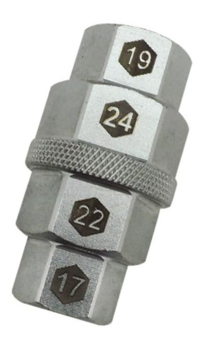
• Use with 3/8" SQ. DR. on both ends and Hex wrench. This tool will allow you to remove the front wheel on any motorcycle that has a 17mm, 19mm, 22mm & 24mm female hex.
