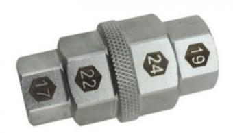
• Use with 3/8" SQ. DR. on both ends and Hex wrench. This tool will allow you to remove the front wheel on any motorcycle that has a 17mm, 19mm, 22mm & 24mm female hex.
