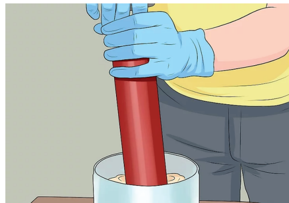
4b. Position the barrel of the gun over a tub of grease. draw back handle 5cm / 2", fill and repeat.
